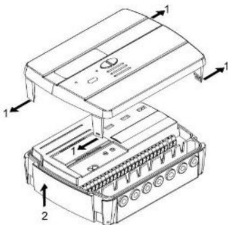
Remove the bracket behind of the calculation unit and secure it to the wall. There are two types of wall mounting allowed:
